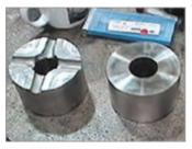
Roughing is done with a 1/2 inch (12.7 mm) Millstar carbide ball insert tool with stiff carbide shank and V-brazed tool head. The shank is held in a shrink-fit adapter. Cutting strategy is Z-level back and forth along the length of the half-round channels, inside-outside pattern, and ramp engage.
